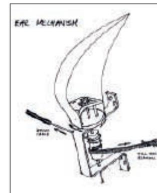
to move through at least 180 degrees, pointing forward they show interest, pointing backwards they indicate fear or alarm, and to the side they show attentiveness. The solution came to me early one morning: mount the ears on short vertical axles, around which would be wound a cable, with a spring to pull the axle back into place and rewind the string. The manipulating finger may only pull through 90 degrees, but the shorter circumference of the axle would give double that for the ear.
